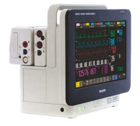
Whether moving a patient throughout the hospital or stationary at bedside, you won't have to bother with adjusting the illumination. The display, with its ambient light sensor, automatically adjust the screen brightness, to maintain readability in nearly any lighting environment.
