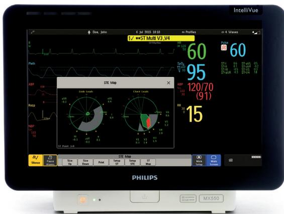
Whether you are examining the patient in a brightly lit environment or allowing the patient to rest with room lights dimmed, you won't have to adjust the monitor's display brightness. The display, with its ambient light sensor, automatically adjusts screen brightness to maintain readability in nearly any lighting environment.
